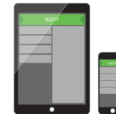
Status changes to orders and machines are reflected instantly in CIMCO Scheduler. When an operator starts work on an order, an indicator turns green and different progress bars show the status of operation, material availability, and delivery. Status information can also be directed to TV screens for open space monitoring and digital signage.
